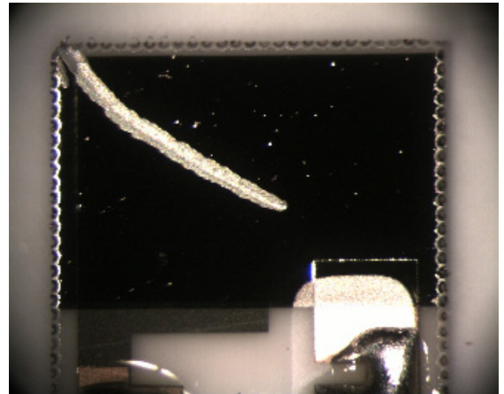
Sensor with a scratch
