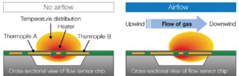
The D6F MEMS sensor chip features two sets of thermopiles located on either side of a tiny heater element. They measure the deviations in heat symmetry caused by gas flowing in either direction. A thin layer of insulating film protects the sensor chip from exposure to the gas.
