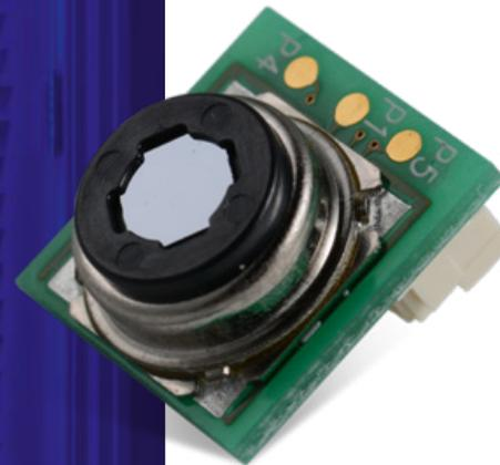
*The D6T miniature non-contact sensor is created entirely from Omron's own ASICs and MEMS technology along with other application-specific parts to ensure high sensitivity. It measures temperature by receiving energy radiated from target objects on thermopile elements.*
