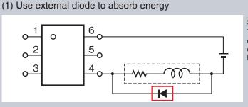
Selection guideline: The reverse breakdown voltage of the diode must be 10 times higher than the
