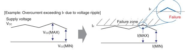
Input ripple voltage must be considered to avoid exceeding the absolute maximum rated value of the LED forward current ( $I_F$ ).
