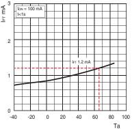
The input current must be designed based on the maximum value of the trigger LED forward current and taking into account the changes in ambient temperature.
