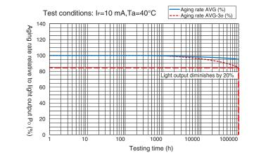
The input current must be designed based on the maximum rating of the LED forward operation current ( $I_{FT}$ ) and must take into account the decline in the LED light output associated with the operating time.
