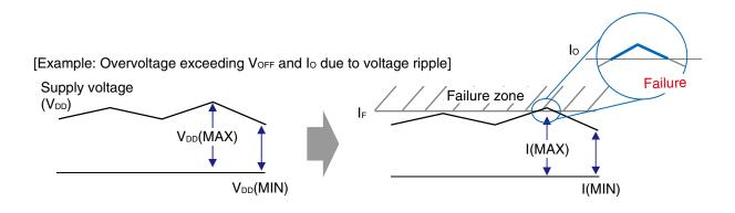
Output ripple voltage must be considered to avoid exceeding the absolute maximum rated values of load voltage ( $V_{OFF}$ ) and continuous load current ( $I_0$ ).
