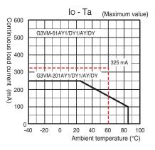
Please make sure to check the continuous load current rates in relation to ambient temperature specified for each model by referring to the Graph: *Continuous Load Current with Ambient Temperature* and select a suitable MOSFET relay (with safety margin) to make sure the product is used under the allowable room temperature of the relay.
