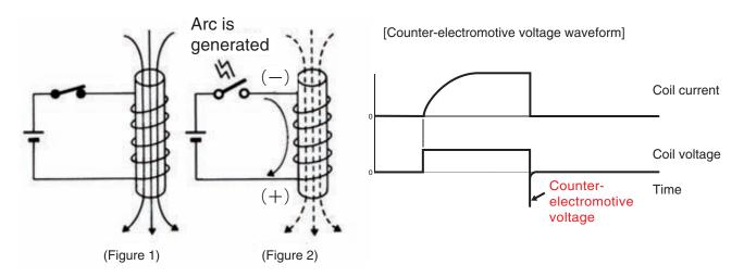
Example) Inductive loads with counter-electromotive force Solenoid, electromagnetic valve, motor brakes, contactors, and mechanical relay etc.
