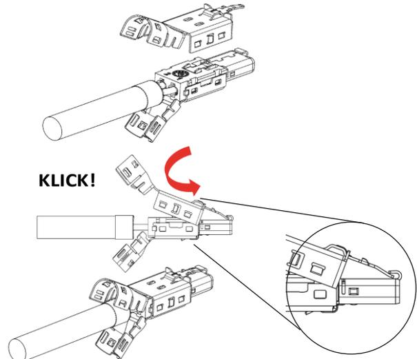
6.7 Bend the lower shielding plate upwards.
