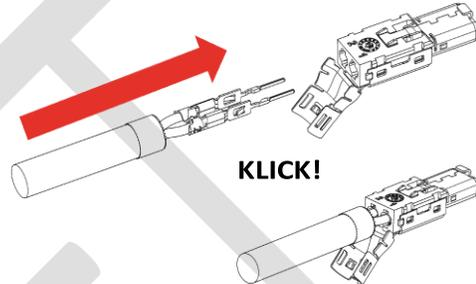
6.5 Check whether the snap-in hooks of the contacts are securely locked in the insulating body. Check window cavity as seen in picture below in circled area.
