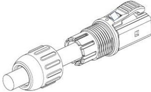
6.2 Strip the cable sheath to a length of 10 mm. Fold the braid back and shorten it to a length of approx. 5 mm. Strip three individual wires to a length of 3 mm.
