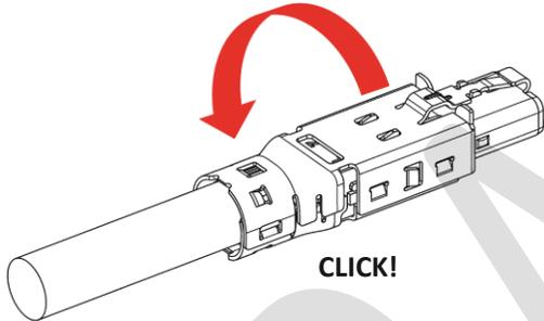
6.9 Slide the connector housing over the mounted data module until it stops. Then tighten the cable gland on block.
