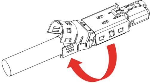
6.8 Bend the upper shielding plate downwards over the lower shielding plate until it locks with an audible “click”. There are two locking levels depending on the cable diameter,
