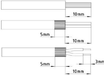
We recommend the use of a tinned copper foil to fix the braided shield.
