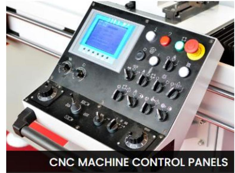
CNC machines use various control interfaces such as working mode selection or speed selection. Our panel-mount potentiometers features a mechanical packages where the rotary movement can be combined with robust detent mechanisms to obtain a high number of mechanical stops.
