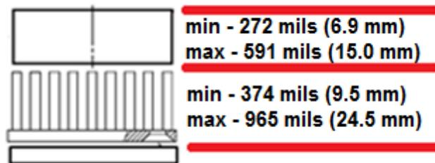
Figure 30 – UltraZed-EV SOM Fan and Heatsink MIN/MAX Combinations
