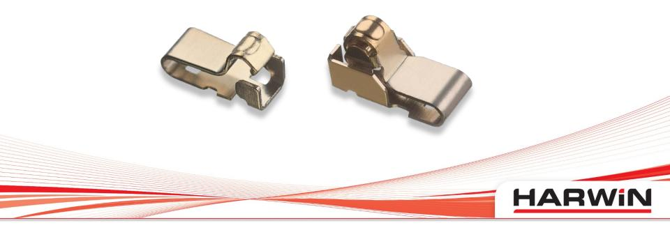
A further development of the extended 'C' style, these contacts were originally designed for wireless antenna connections on many mobile devices, such as smartphones, or LED lamp connection and RFID tags. The Positive Stop shoulder prevents the contact from being over-compressed, which can lead to permanent set and a reduction in spring force. This range is all ultra-low profile, with 6 contacts ranging from just 1.23mm to 2mm high.
