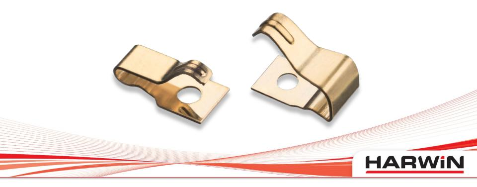
A development of the 'C' style contact, this design uses a more obvious cantilever style. The SMT pick and place area is exaggerated to compensate for the miniature size of the contact. This range is provided in 0.5mm incremental step heights, from 2mm up to 5mm. The footprint is the same across the complete set of contacts.
