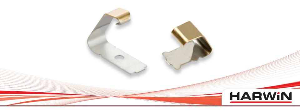
The 'C' style contact is the simplest of designs, providing a flexible connection between PCBs, components and chassis grounds. Manufactured from copper alloy, they provide excellent spring properties over extended periods of time. Harwin provide a choice of 6 different parts in this style, with heights ranging between 1.7mm to 5.5mm.
