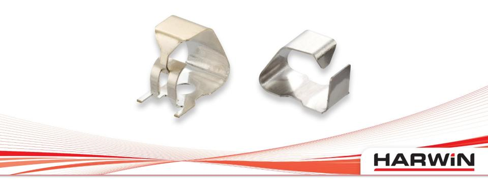
'Box' style contacts are different to the 'C' style by the addition of a feature that reduces the risk of damage caused by 'accidental snagging'. On some Box designs, it also prevents unwanted lateral movement of the contact during mating. Typical applications are identical to the 'C' style contacts. The 'Box' style contacts are available in 5 different heights from 2.5mm to 6mm.
