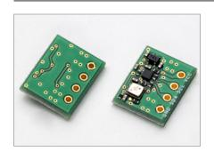
This evaluation board will support you when checking and studying the function and performance of our barometric pressure sensor (ZPA2326-0311A). This is a capacitive type MEMS device, combined with ASIC incorporating an I2C interface. As its voltage level is 1.8V, this board includes a level converter which enables the user to connect directly to 3.3V system. Via I2C, we can also obtain information about the barometric pressure and temperature.
