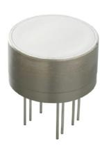
The FR sensor uses a semiconductor MR element (SMR) and a permanent magnet. It outputs a para-sine wave depending on the turn and movement of the ferromagnetic gear or rack which it faces.
