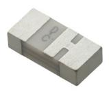
The shock sensor detects vibration or acceleration induced as a result of shock and generates electrical charges which are proportional to the applied acceleration. The core technology is piezoelectric ceramic and applications include predictive maintenance, and a range of consumer applications including hard disc drives, gaming devices and digital photo frames.
