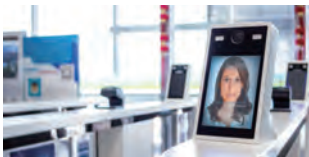
Access Control System/ Speed Gate
