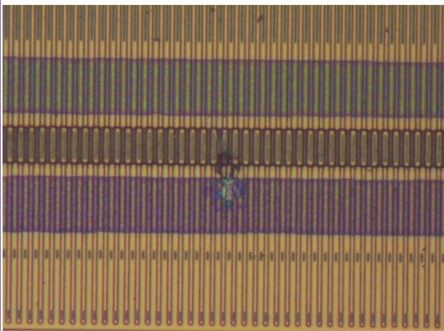
Figure 16. Device 4 after Al removal
