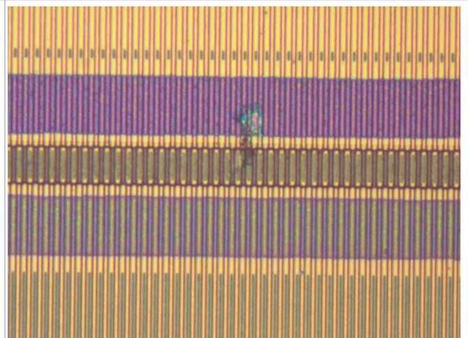
Figure 21. Device 3 after Al, barrier and TEOS etch
