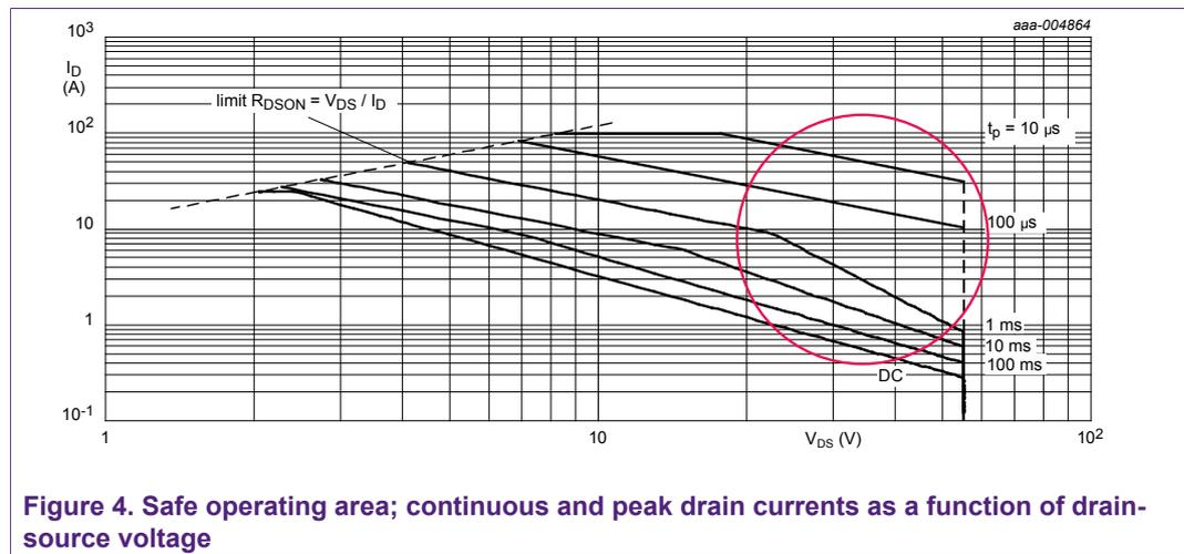
Figure 4. Safe operating area; continuous and peak drain currents as a function of drain-source voltage
