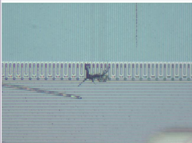
Figure 20. Device 2 after Al, barrier and TEOS etch
