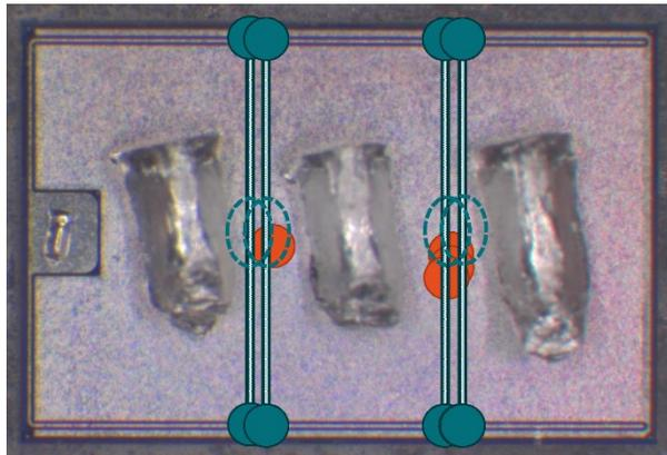
Failure signature of electrical overstress on power MOSFETs
