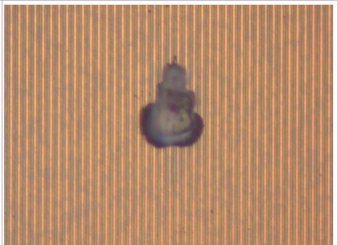
Figure 38. Device 4 lower (orange) hotspot
