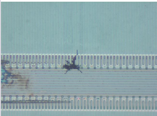
Figure 22. Device 4 after Al, barrier and TEOS etch
