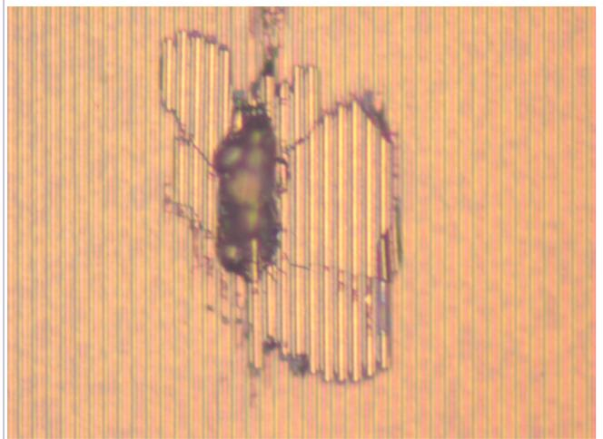
Figure 36. Device 1 lower (orange) hotspot
