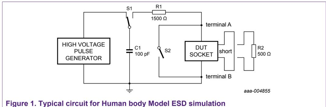
Figure 1. Typical circuit for Human body Model ESD simulation
