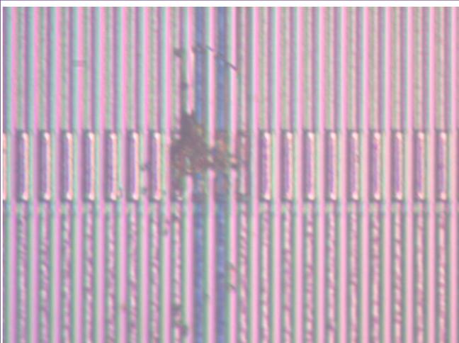
Figure 18. Device 5 after TEOS removal
