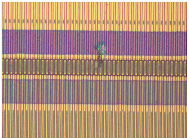
Figure 17. Device 7 after Al removal
