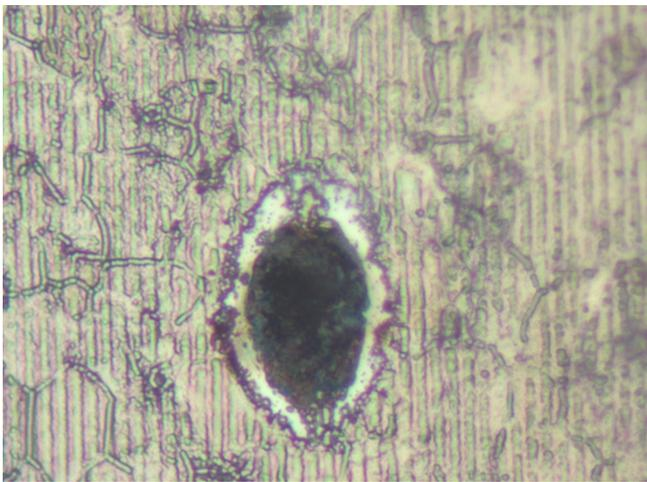
Figure 74. Device 5 upper (orange) hotspot
