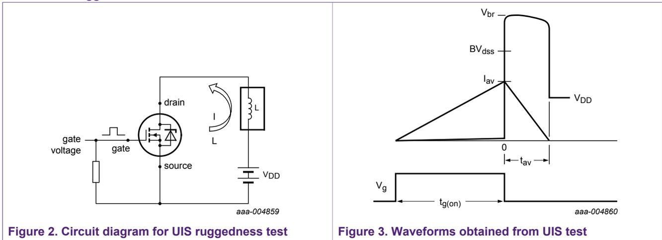
1.2.2 Fault condition simulated
