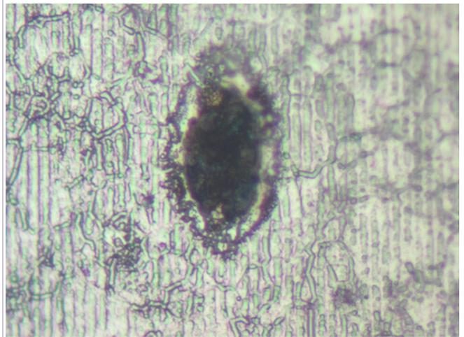
Figure 75. Device 6 lower (orange) hotspot
