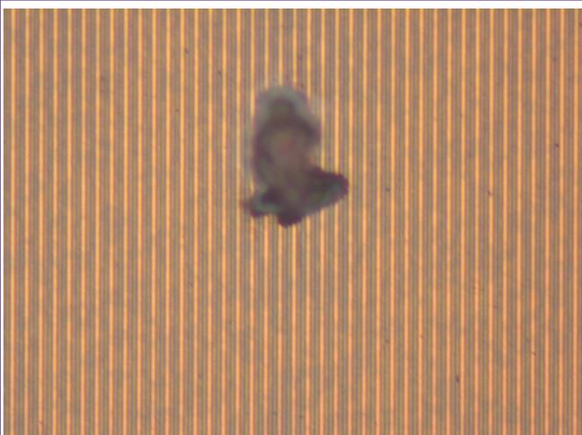
Figure 37. Device 4 upper (orange) hotspot
