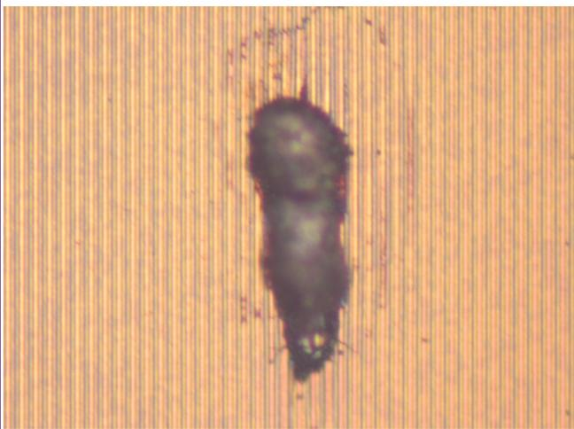
Figure 35. Device 1 upper (orange) hotspot
