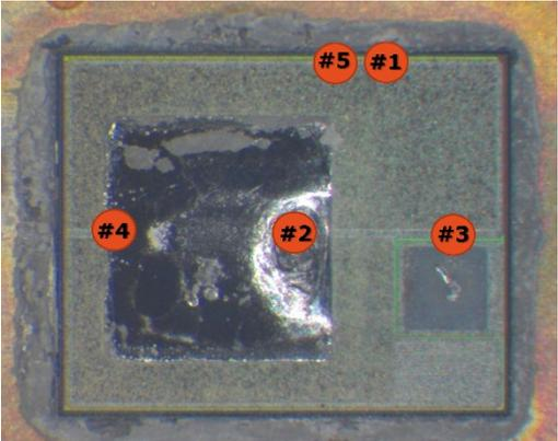
A scanning electron micrograph (SEM) of a MOSFET die. The die is square-shaped with a central gate region. Five red circles with black text labels (#1 through #5) are placed on the die to indicate specific failure sites. #1 and #5 are at the top edge, #2 is in the central gate region, #3 is on the right edge, and #4 is on the left edge.
