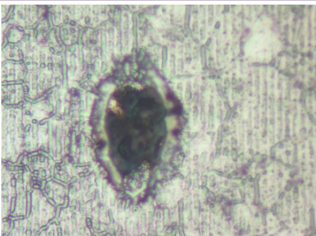
Figure 76. Device 7 upper (orange) hotspot
