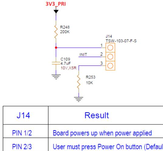
**Figure 3 – Board INIT Header**
