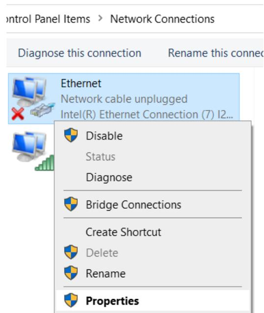
Figure 13 – Ethernet Adapter Properties
