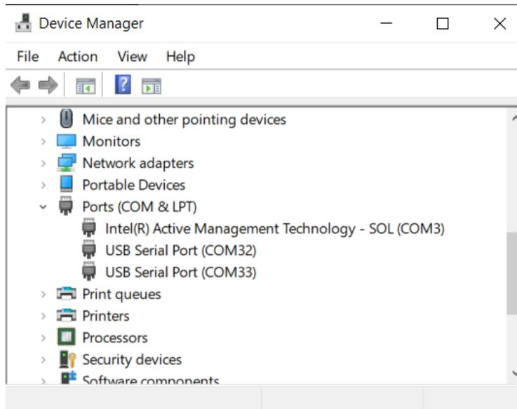
**Figure 8 – USB-JTAG/UART COM Port Assignments**
