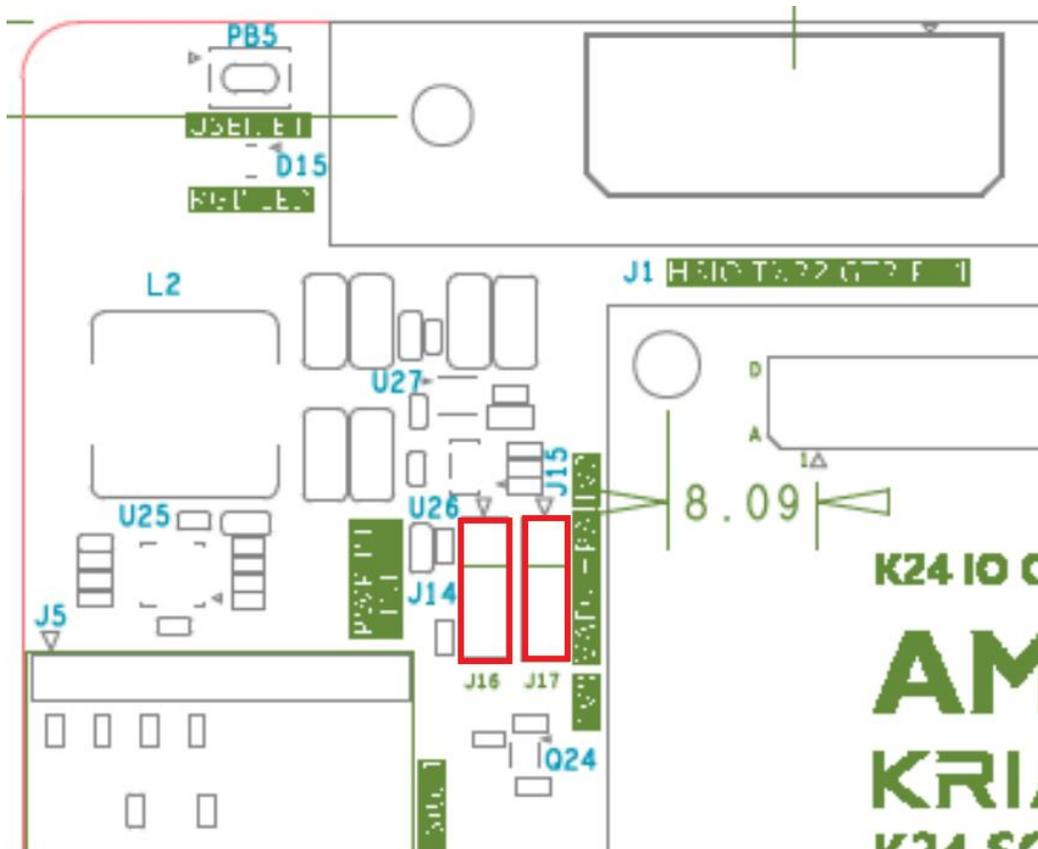
**Figure 5 – Header Locations on Carrier Card**
