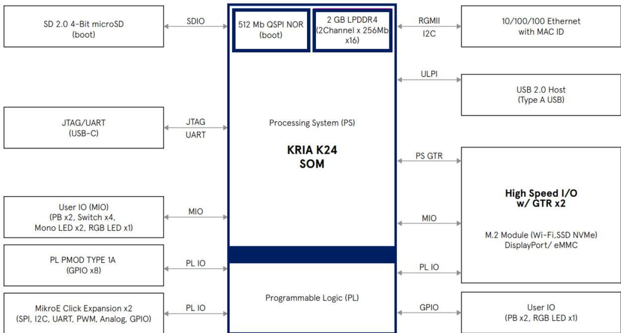
**Figure 1 – Development Kit Block Diagram**
