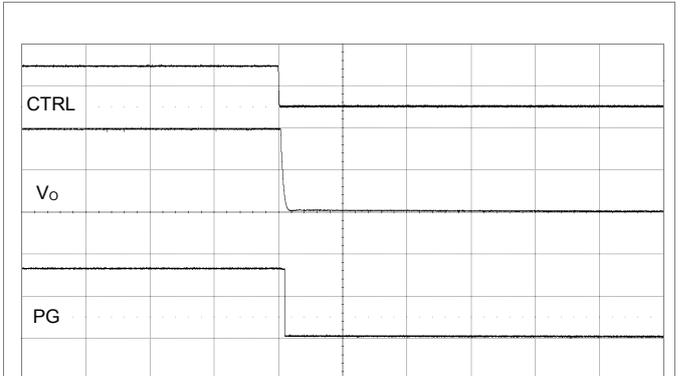
Output disabled by CTRL pin.  $V_i = 12\text{ V}$ ,  $I_o = \text{max } I_o$ .
