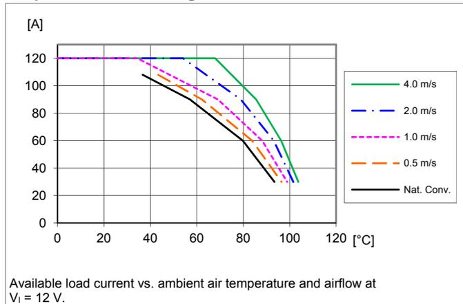
**Output Current Derating for Lay Down versions**
