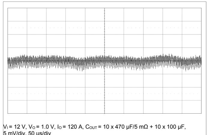
$V_i = 12\text{ V}$ ,  $V_o = 1.0\text{ V}$ ,  $I_o = 120\text{ A}$ ,  $C_{OUT} = 10 \times 470\text{ µF}/5\text{ m}\Omega + 10 \times 100\text{ µF}$ ,
