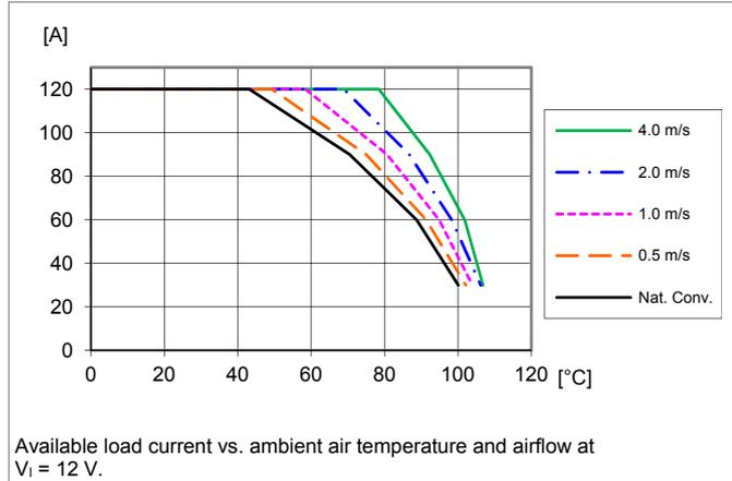
**Output Current Derating for Lay Down versions**
