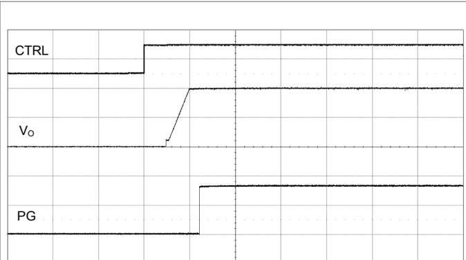
Output enabled by CTRL pin.  $V_i = 12\text{ V}$ ,  $I_o = \text{max } I_o$ .
