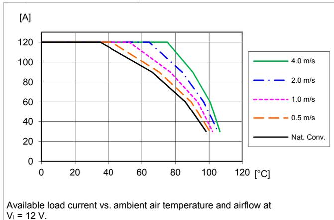
**Output Current Derating for Lay Down versions**
