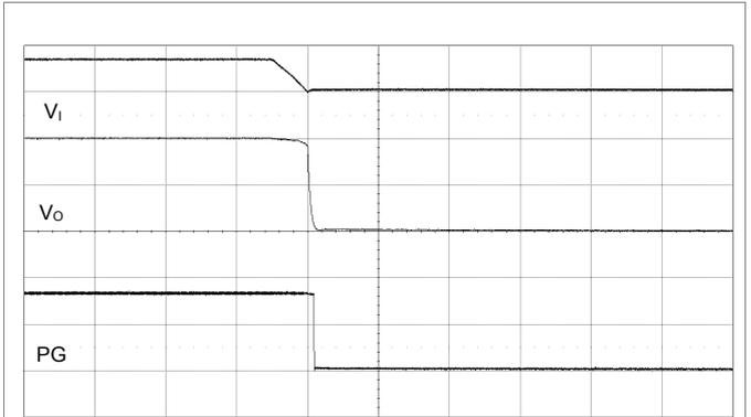
Output disabled by removing  $V_i$ .  $V_i = 12\text{ V}$ ,  $I_o = \text{max } I_o$ .
