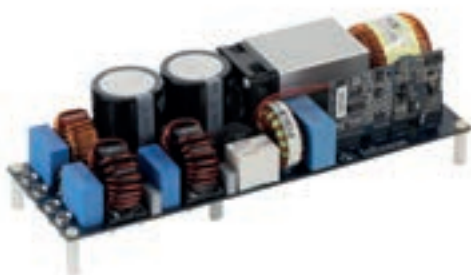
2.5 kW totem pole PFC board: EVAL_2500W_PFC_GAN_A
