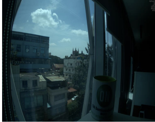
Figure 1. Image with Shorter Exposure Time Captures Detail in the Bright Areas and Loses Detail in the Dark
