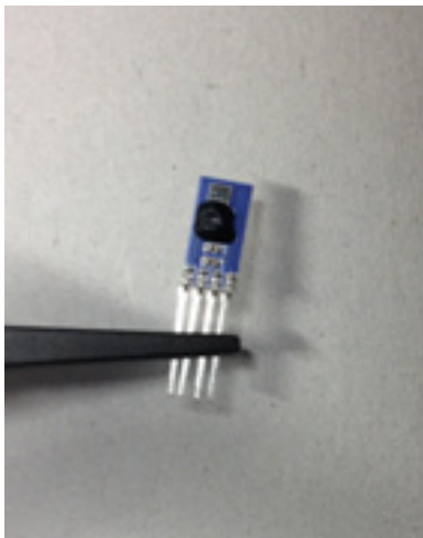
Sensor held with plastic tweezers on the wires only
