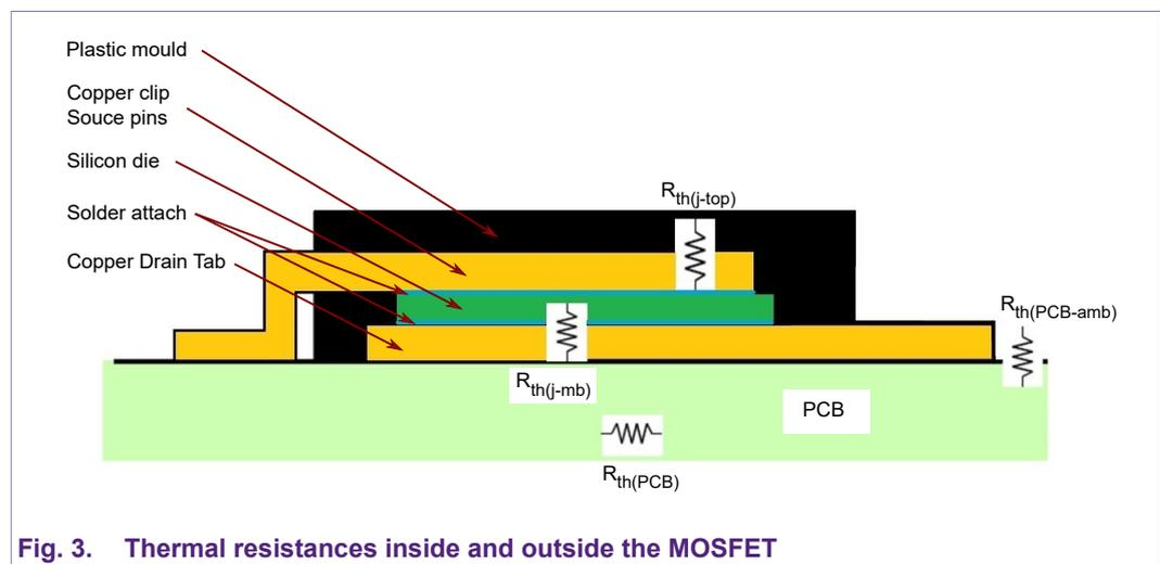
**Fig. 3. Thermal resistances inside and outside the MOSFET**
