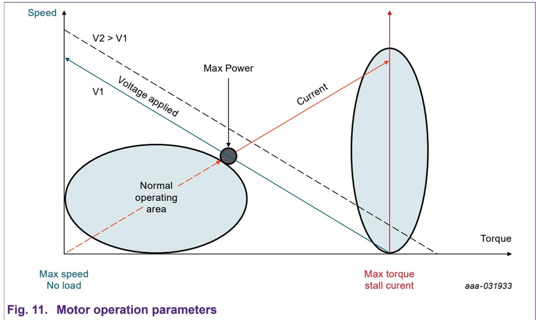
**Fig. 11. Motor operation parameters**
