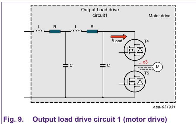
Fig. 9. Output load drive circuit 1 (motor drive)
