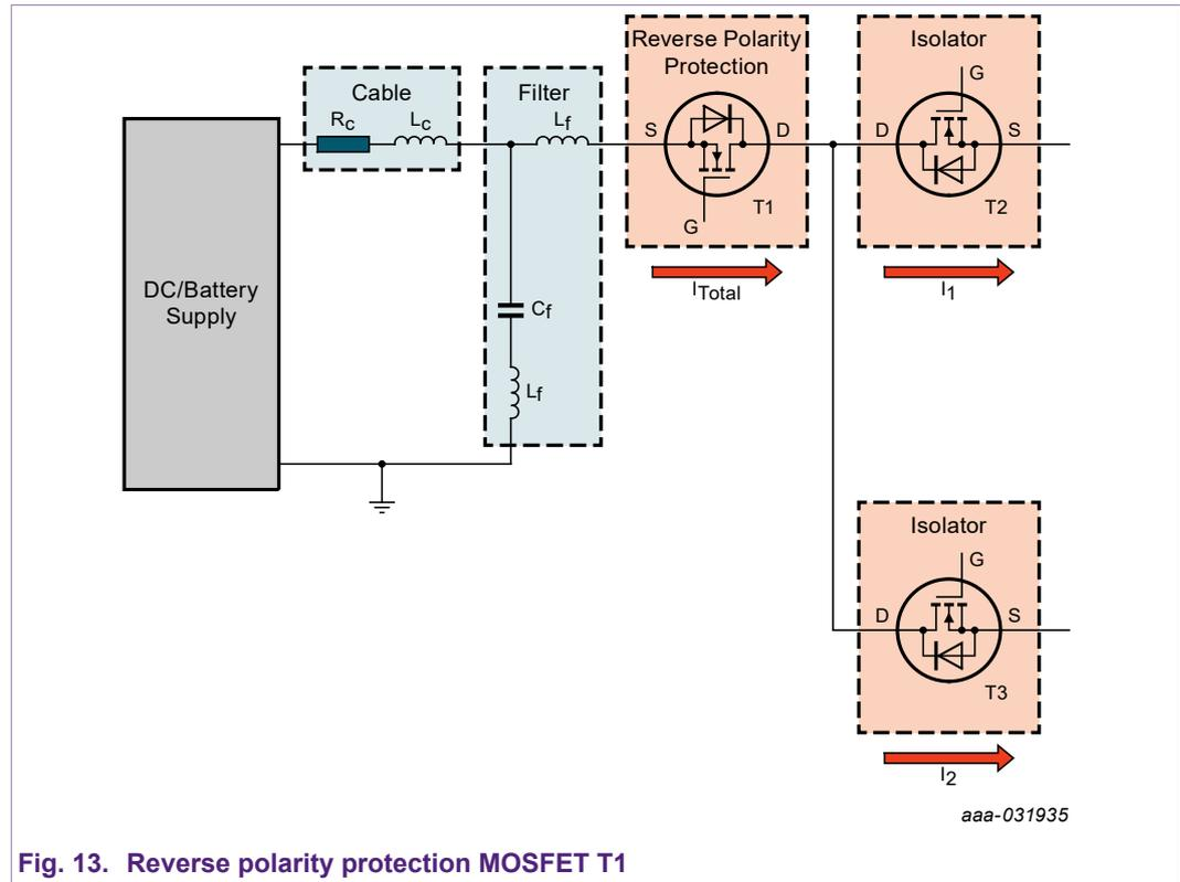
Fig. 13. Reverse polarity protection MOSFET T1
