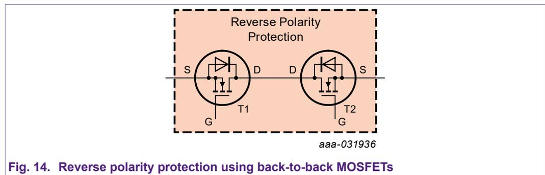
Fig. 14. Reverse polarity protection using back-to-back MOSFETs
