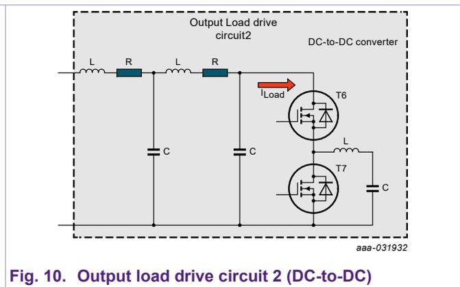
Fig. 10. Output load drive circuit 2 (DC-to-DC)
