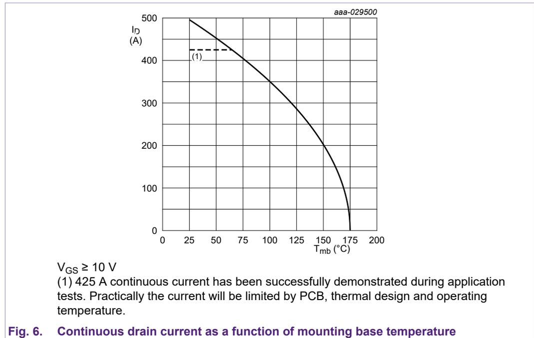
**Fig. 6. Continuous drain current as a function of mounting base temperature**
