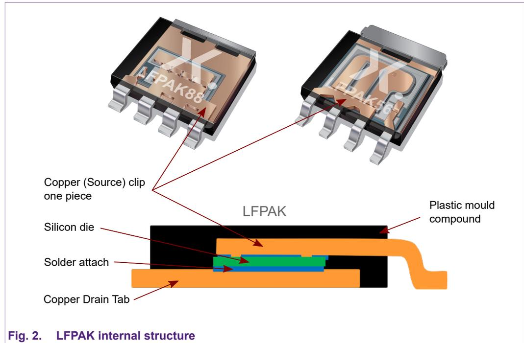
Fig. 2. LFLPAK internal structure
