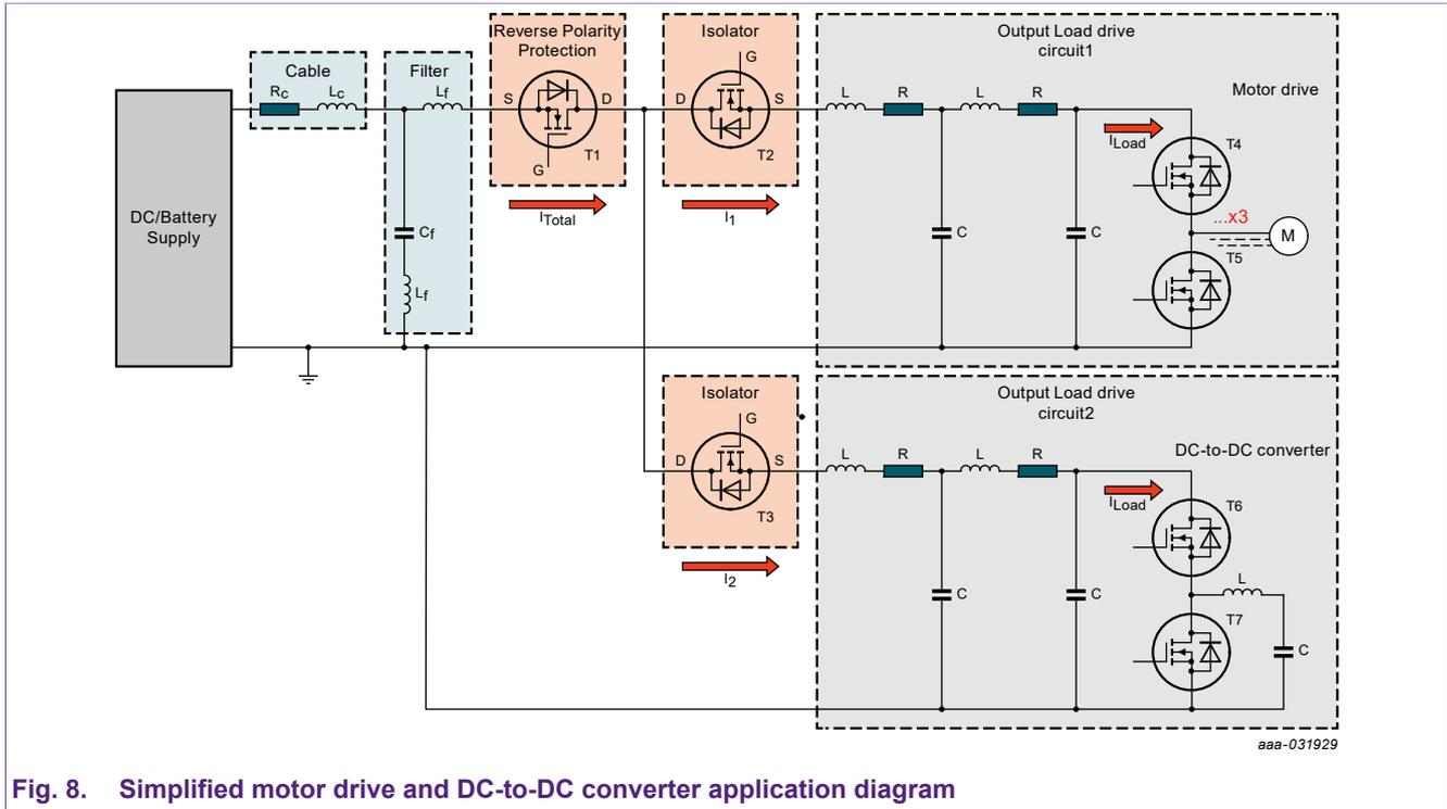
Fig. 8. Simplified motor drive and DC-to-DC converter application diagram
