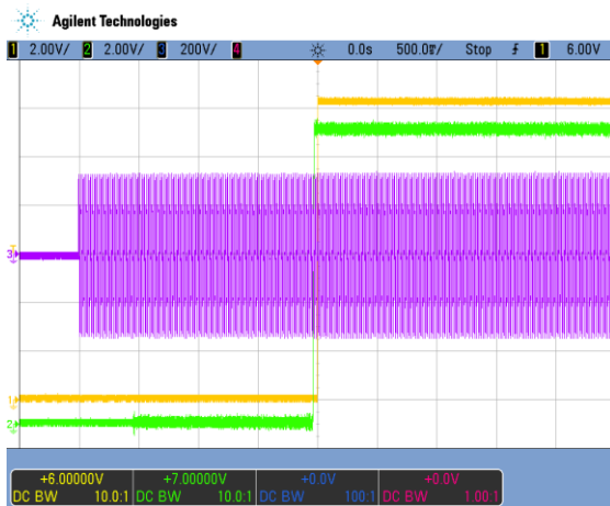
Figure 7 - Turn-On AC Line 230 VAC, full load (500 ns/div) CH1: V1 (2 V/div); CH2: VSB (2 V/div); CH3: Vin (200 V/div)
