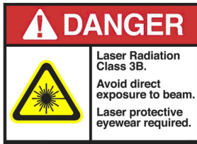
Figure 7: Laser Safety Warning Sign for Unrecommended/Non-Default Operation
