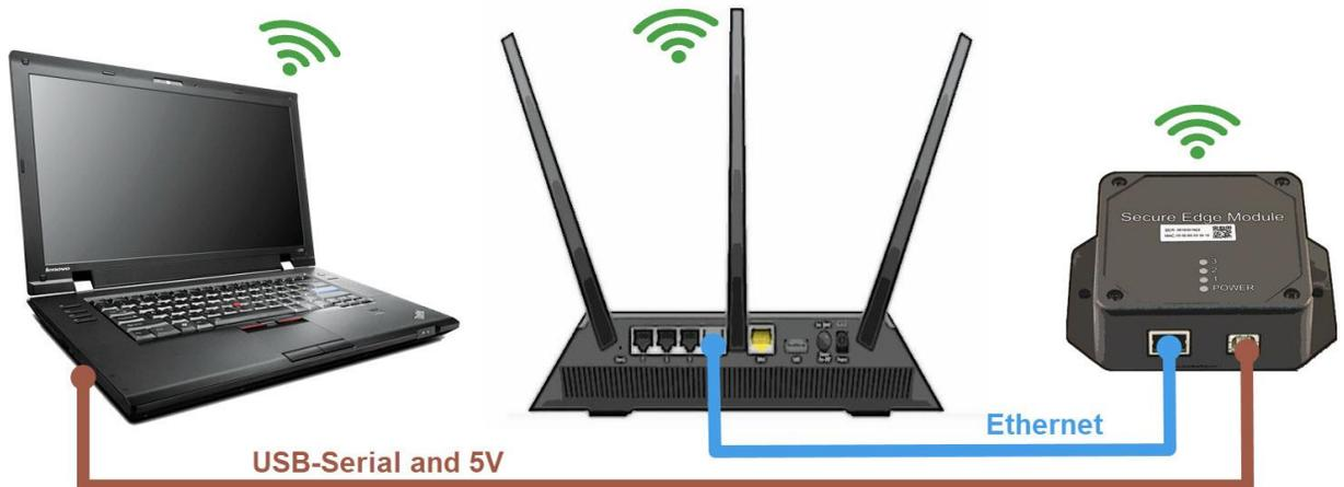
**Figure 8 – Hardware Test Setup**
